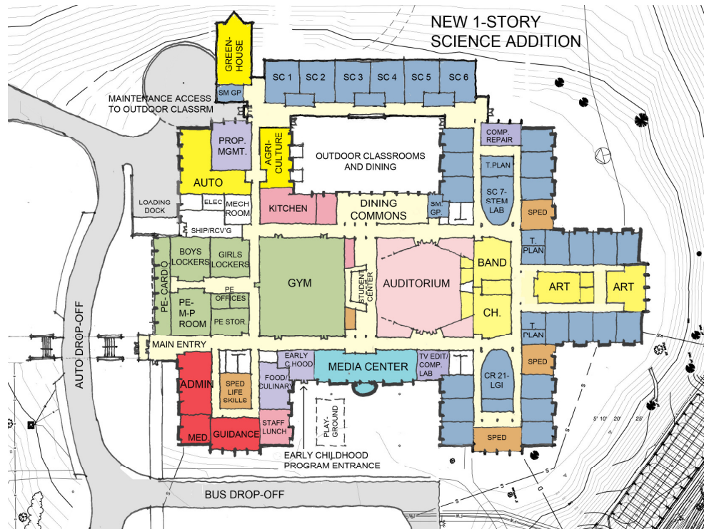
OPTION 2D.4 – One-story, new construction east of the MMRHS. The spaces are color coded based on colors designated on the Proposed Space Summary.
